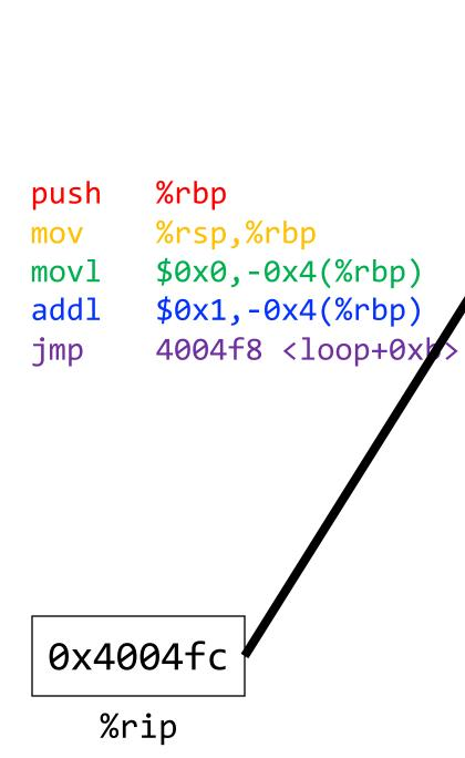
4004fd fa 4004fc eb 4004fb **01** fc 4004fa 4004f9 45 4004f8 83 4004f7 00 4004f6 00 4004f5 00 4004f4 00 fc 4004f3 45 4004f2 4004f1 **c7** 4004f0 **e5** 89 4004ef 4004ee 48 55 4004ed
