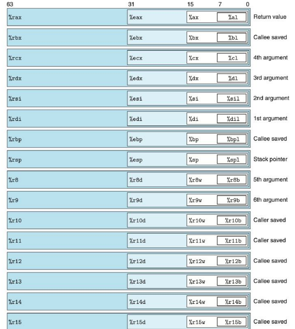
Figure 3.2 Integer registers. The low-order portions of all 16 registers can be accessed as byte, word (16-bit), double word (32-bit), and quad word (64-bit) quantities.
