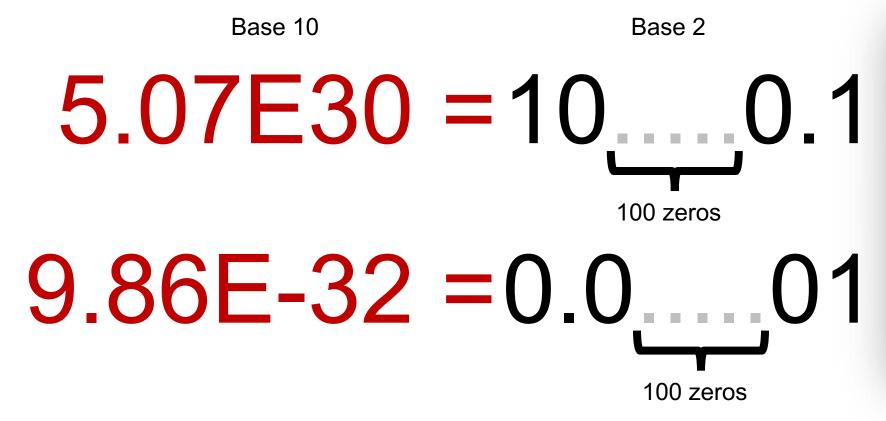
To be able to store both these numbers using the same fixed point representation, the bitwidth of the type would need to be at least 207 bits wide!
