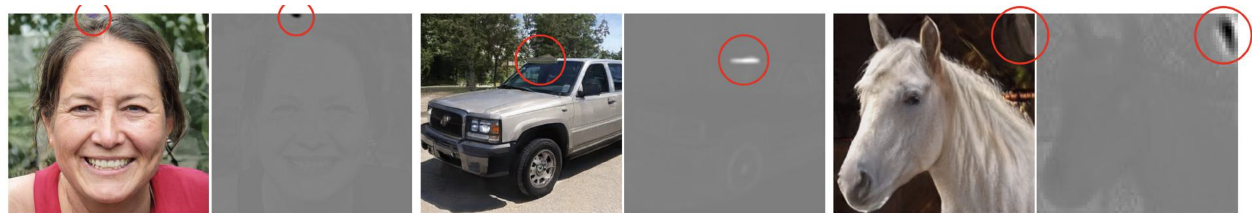
Figure 1. Instance normalization causes water droplet -like artifacts in StyleGAN images. These are not always obvious in the generated images, but if we look at the activations inside the generator network, the problem is always there, in all feature maps starting from the 64x64 resolution. It is a systemic problem that plagues all StyleGAN images.
